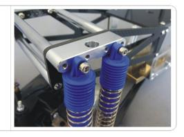
The Stock Plus chassis has the same suspension mounting points as the original plastic tub. You will need the ball joints from the original chassis to mount your gearboxes and ladder bars.
