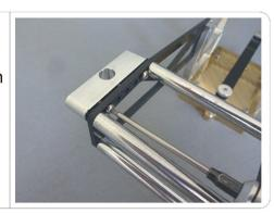
Driver access is hampered so tighten with a 2.5mm allen key.
